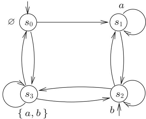
Switching function:  $\Delta(\underbrace{x_1, x_2}_{s}, \underbrace{x'_1, x'_2}_{s'}) = 1$  if and only if  $s \rightarrow s'$
