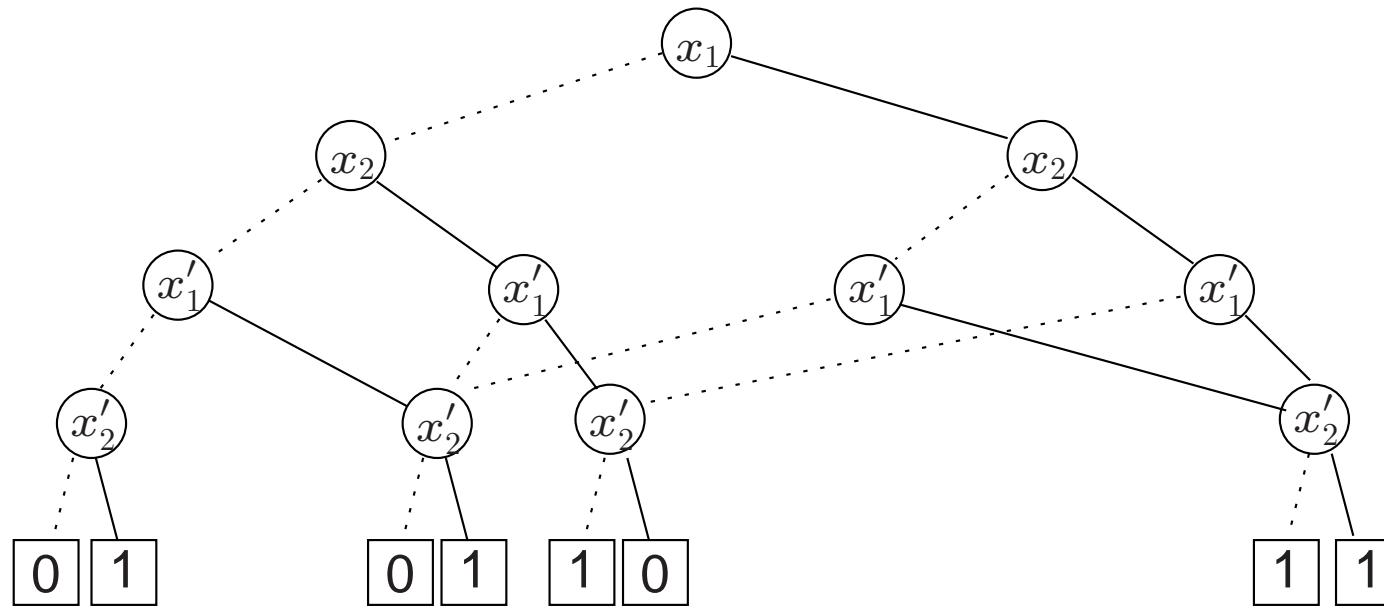
An example OBDD representing  $f_>$  for our example using  $x_1 < x_2 < x'_1 < x'_2$
