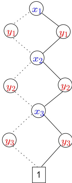
The ROBDD of  $f_{stab}(\bar{x}, \bar{y}) = (x_1 \leftrightarrow y_1) \wedge \dots \wedge (x_n \leftrightarrow y_n)$
