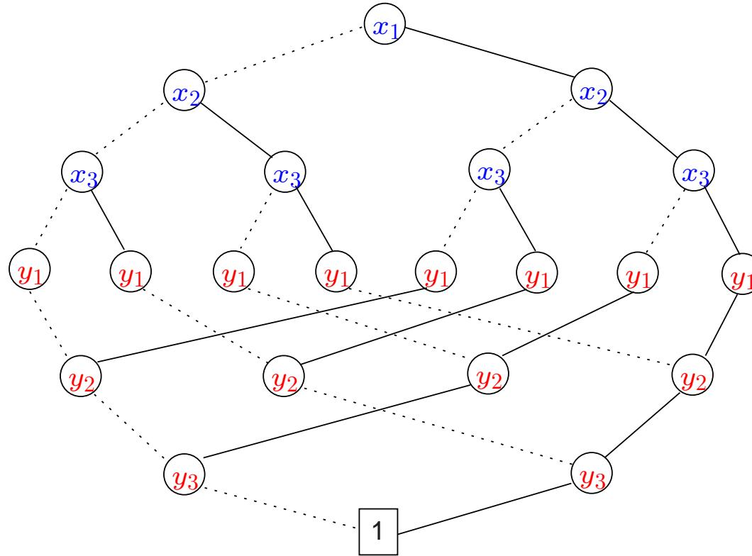
The ROBDD of  $f_{stab}(\bar{x}, \bar{y}) = (x_1 \leftrightarrow y_1) \wedge \dots \wedge (x_n \leftrightarrow y_n)$
