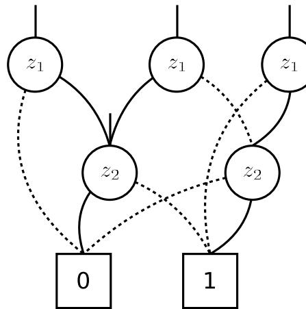
Shared OBDD representing  $\underbrace{z_1 \wedge \neg z_2}_{f_1}$ ,  $\underbrace{\neg z_2}_{f_2}$ ,  $\underbrace{z_1 \oplus z_2}_{f_3}$  and  $\underbrace{\neg z_1 \vee z_2}_{f_4}$
