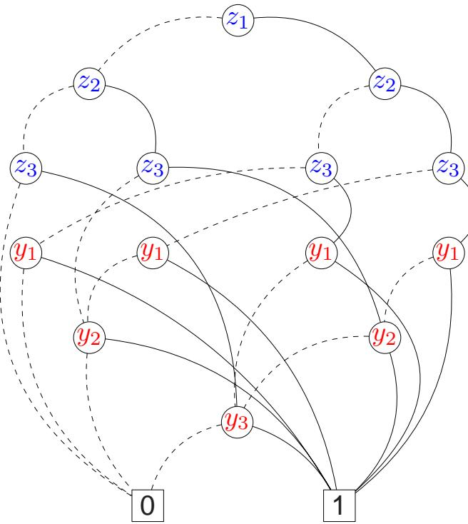
ROBDD for  $f_3(\bar{z}, \bar{y}) = (z_1 \wedge y_1) \vee (z_2 \wedge y_2) \vee (z_3 \wedge y_3)$
