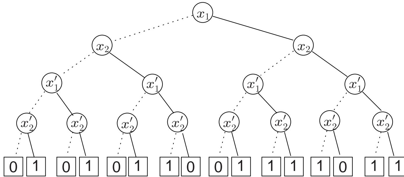
A BDT representing  $f_{\rightarrow}$  for our example using  $x_1 < x_2 < x'_1 < x'_2$
