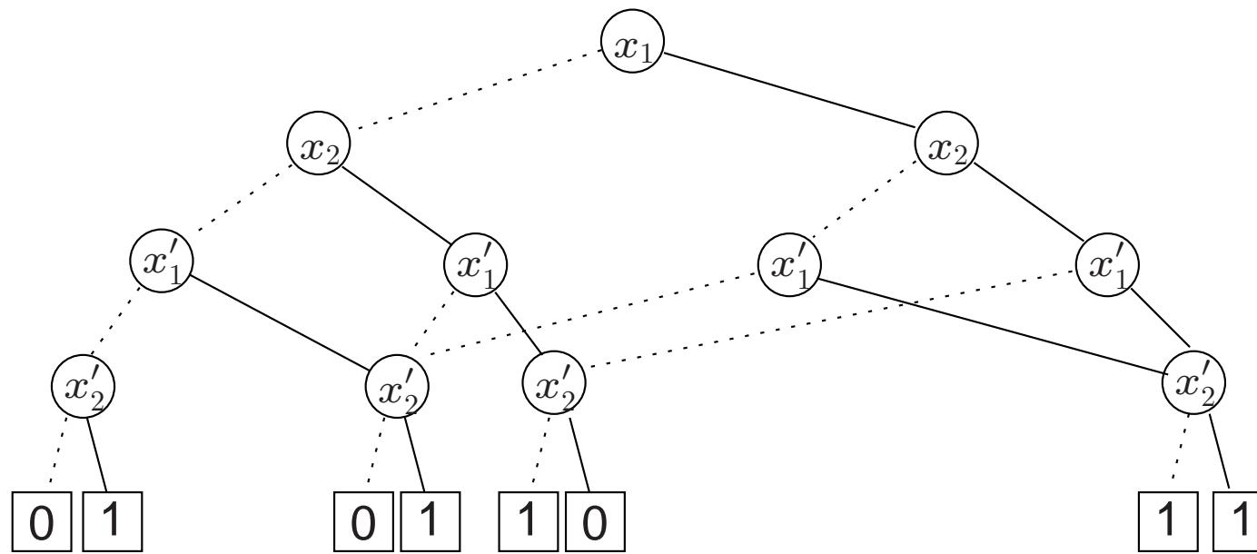
An example OBDD representing  $f_{\rightarrow}$  for our example using  $x_1 < x_2 < x'_1 < x'_2$
