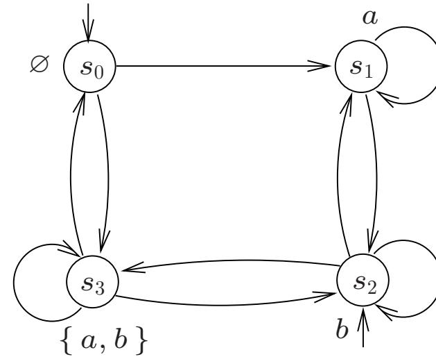
$$\underline{i} = \begin{pmatrix} 1 \\ 0 \\ 1 \\ 0 \end{pmatrix} \quad \text{and} \quad \mathbf{T} = \begin{pmatrix} 0 & 1 & 0 & 1 \\ 0 & 1 & 1 & 0 \\ 0 & 1 & 1 & 1 \\ 1 & 0 & 1 & 1 \end{pmatrix} \quad \text{and} \quad \mathbf{L} = \begin{pmatrix} 0 & 0 \\ 0 & 1 \\ 1 & 0 \\ 1 & 1 \end{pmatrix}$$
