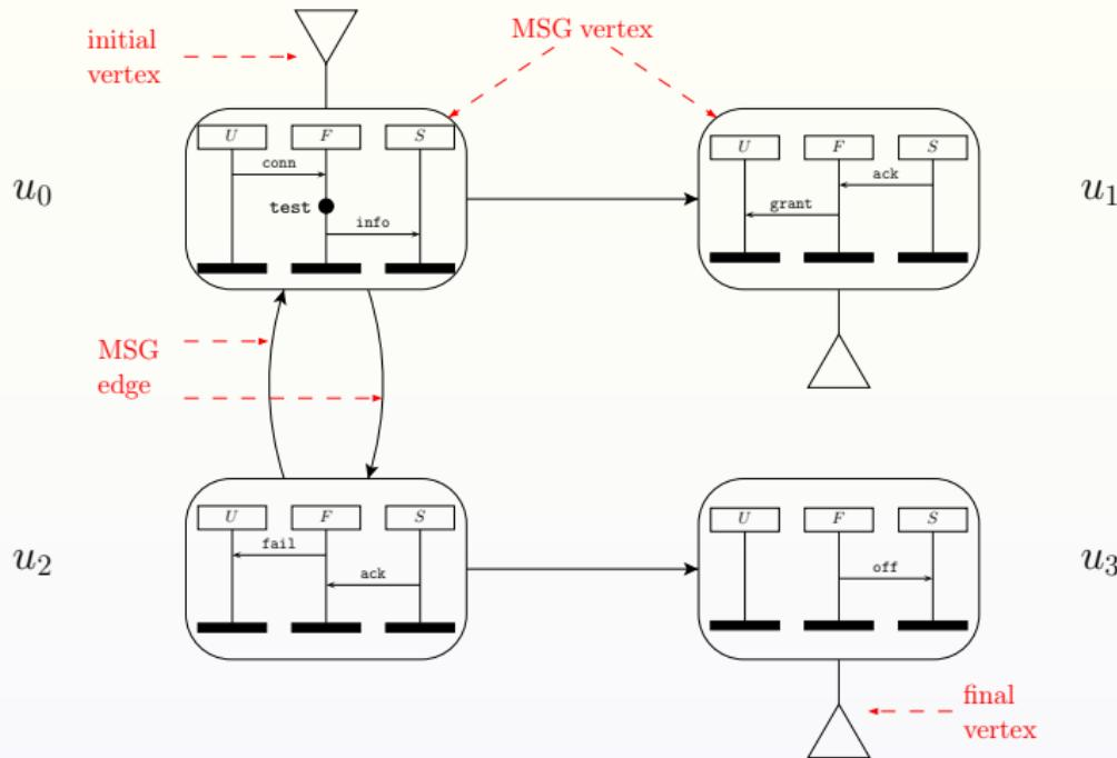
$\underbrace{u_0 \ u_2 \ u_0 \ u_1}_{\text{path in graph}} \text{ yields } \underbrace{\lambda(u_0) \bullet \lambda(u_2) \bullet \lambda(u_0) \bullet \lambda(u_1)}_{\text{MSC of the path}}$
