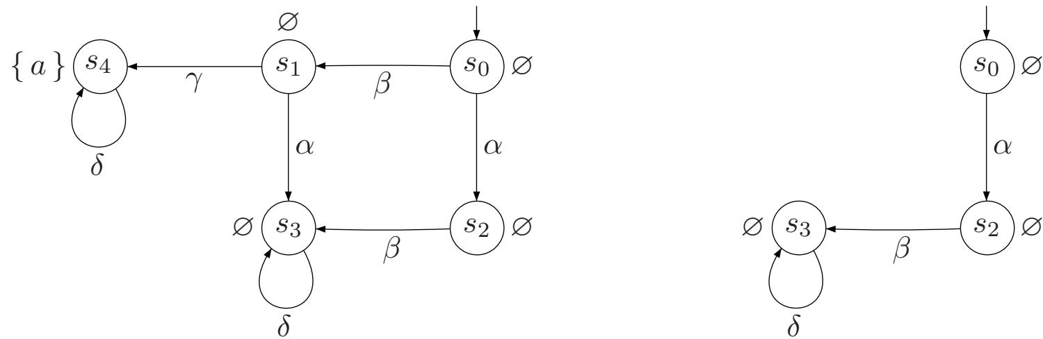
run  $s_0 \xrightarrow{\beta} s_1 \xrightarrow{\gamma} s_4$  violates (A2) as  $\gamma$  depends on  $\alpha \in \text{ample}(s_0)$
