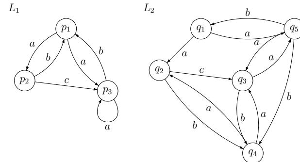
Let  $S = \{p_1, \dots, p_3, q_1, \dots, q_5\}$ . Show that  $p_1 \sim_B q_1$ , i.e., find a bisimulation relation  $R \subseteq S \times S$  with  $p_1 R q_1$ .
