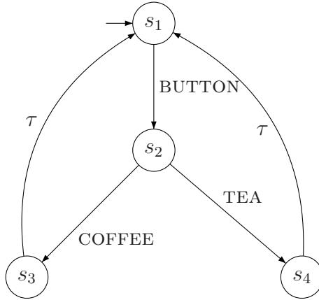
Not that an LTS is similar to a (finite) automaton. However, the difference here is that we usually do not have a starting state, and also no accepting states.
