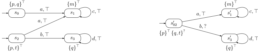
Figure 3.3: The MTS M (left) is abstracted by the MTS M' (right), i.e., M' = \alpha(M)
