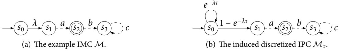
Figure 6.3: Interval and time-bounded reachability in IMCs.
